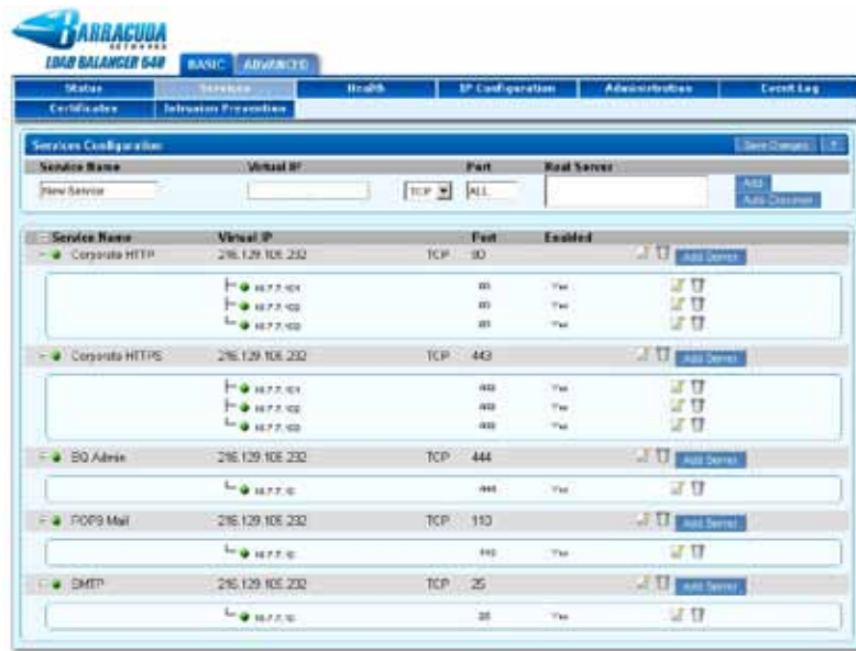
The Barracuda Load Balancer distributes traffic for multiple services, including Web, email and other network applications.
